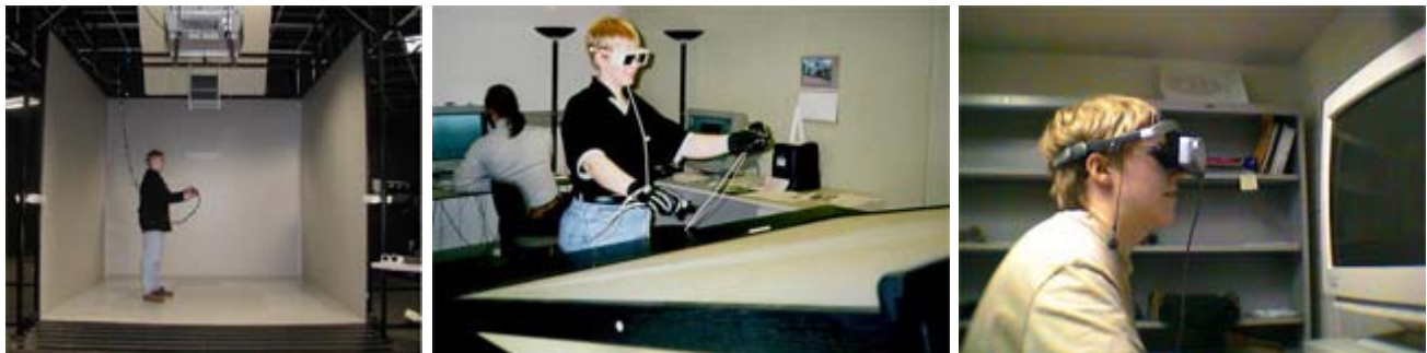
Figure 2: (a) User in a CAVE-like immersive, virtual environment (COVE system at the Engineering Research Center at Mississippi State University) and using a (b) Virtual Workbench and (c) a Head Mounted Display (HMD)
