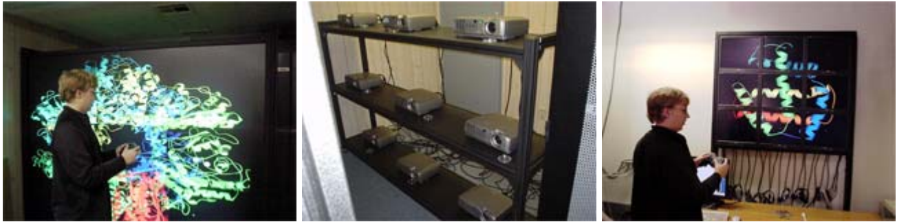
Figure 3: (a) and (b) Tiled 3x3 Projector Display with 9 projectors, (c) Tiled 3x3 LC Display
