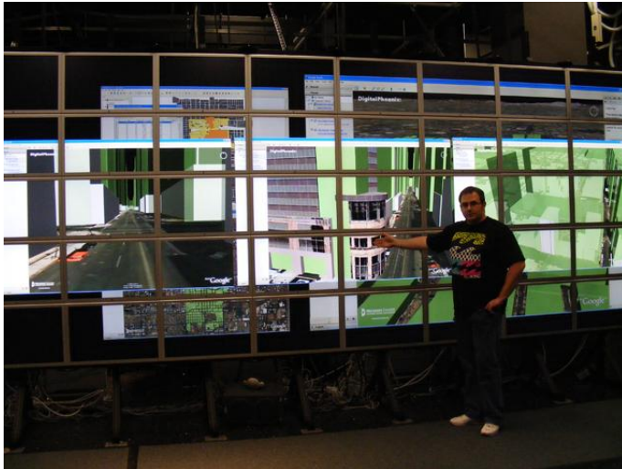
Figure 10: HIPerWall: Violations shown with overlay of existing buildings and visualization consistent with building code. For better visibility transparency can be added. Multiple windows can be examined and analyzed by multiple users.
